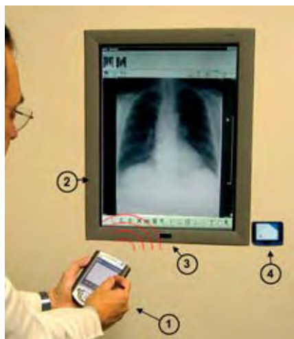
Fig. 2: Pocket PC (1) communicates with the flat panel display device (2) via an infrared channel (3). The additional touch pad device (4) is mounted next to the flat panel device for manual image and display functions.
