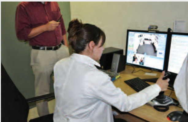
Photo 1. RP-7i® Control Station: Desktop monitor, camera, joystick DT, speakers, keyboard, mouse, microphone and computer. Intensivist at the Maternal and Perinatal University Hospital, Mexico.
