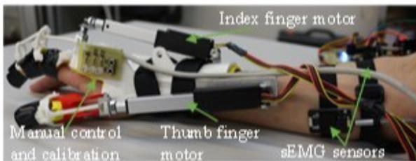
Figure 2: Upper limb exoskeleton example (Farinha et al. 2019)
