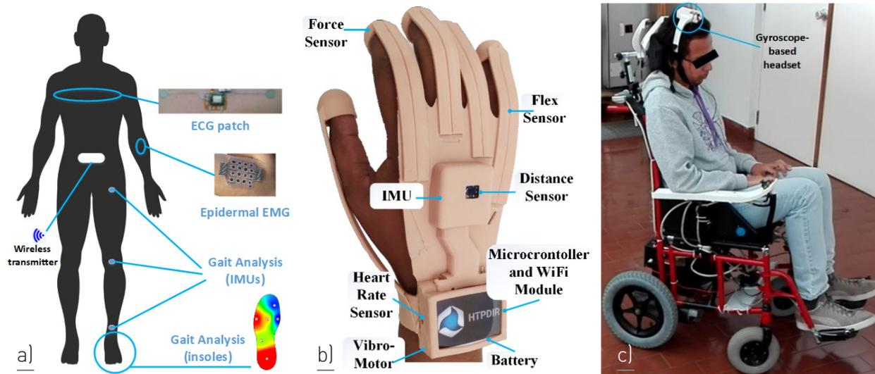
**Figure 1:** Wearable sensors. a) Examples of body sensors for EMG and ECG monitoring and gait and joint motion analysis (using inertial motion units and force sensors); b) Wearable glove designed for hand movements and finger bending, as well as to sense fingertips pressure (Almeida et al. 2019); c) Motion sensors (gyroscopes) used to control a wheelchair with head movement (Gomes et al. 2019).
