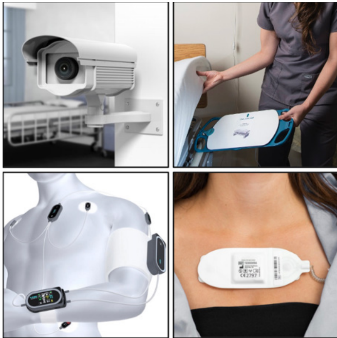
Figure 1. Examples of solutions for continuous monitoring on hospital wards Top = "Stay-in-bed" monitoring with video cameras (left), and piezo electric pad under the mattress (right). Bottom = mobile monitoring with multiple sensors (electrodes, brachial cuff and finger pulse oximeter) (left), and a single wireless adhesive patch measuring heart rate, respiratory rate and axillary temperature (right).
