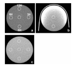
Figure 4. Regions of interest for each material on module 1 in different configurations: (a) without protection (b) with protection and one sponge (c) the protection attached to the gantry
