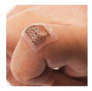
Researchers have combined wireless and ultrasound technologies to develop a wearable patch that can monitor blood pressure (BP) in arteries deep beneath the skin. This ultrasound patch provides an easy way to help people detect cardiovascular problems earlier on and with greater precision. A team of researchers led by the University of California San Diego describe their work in a paper published in Nature Biomedical Engineering.
