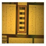
A silicon circuit, coated with a protective layer and immersed in fluid that mimicks human body chemistry. Photo courtesy of Ohio State University.
