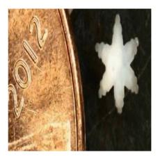
A tiny robotic 'hand' made from flexible, partially biodegradable material could assist physicians with remotely guided surgery, and eventually deliver drugs to parts of the body which are otherwise difficult to reach.
