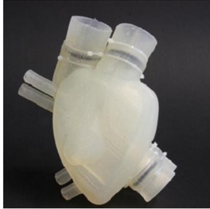
A soft artificial heart that beats almost like a human heart has been developed by researchers from ETH Zurich. The artificial heart was created from silicone using a 3D-printing, lost-wax casting technique; it weighs 390 grams and has a volume of 679 cubic centimetres.
