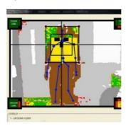
Researchers have developed software for the Microsoft Kinect gaming console that measures body-part thickness and checks for motion, positioning and beam adjustment immediately before x-ray imaging. The goal is to have the best quality x-rays at the lowest dose possible without repeating images, the researchers explained. Their feasibility study was presented on Tuesday, 1 December, at the annual meeting of the Radiological Society of North America (RSNA).
