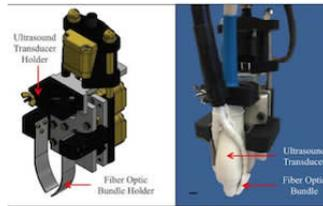
Purdue University researchers are developing a novel biomedical imaging system, known as photoacoustic tomography (PAT), that combines optical and ultrasound technology to improve diagnosis of life-threatening diseases. The system provides real-time compositional information of body tissue without the need for contrast agents and with better depth penetration compared with conventional optical techniques.
