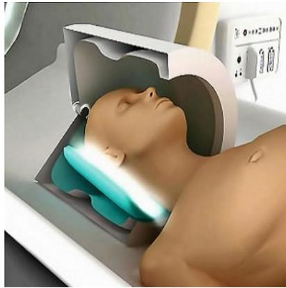
Scientists from Leiden University Medical Center in the Netherlands and ITMO University in Russia have designed and tested a new metasurface-based technology that can enhance the local sensitivity of MRI scanners on humans. This metasurface consists of thin resonant strips that are arranged periodically. When placed under the patient's head, this metasurface provides much higher signals from the local brain region. Details of this new technology are published in Scientific Reports.
