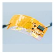
The Spatiotemporal On-Demand Patch's exposed circuit will be covered by material resembling a Band-Aid. It can receive commands wirelessly from a smartphone or computer to schedule and trigger the release of drugs from individual microneedles.
