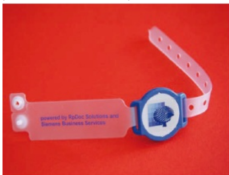
The RFID wristband that has been developed and optimized for patient comfort and acceptance by two commercial project partners.
