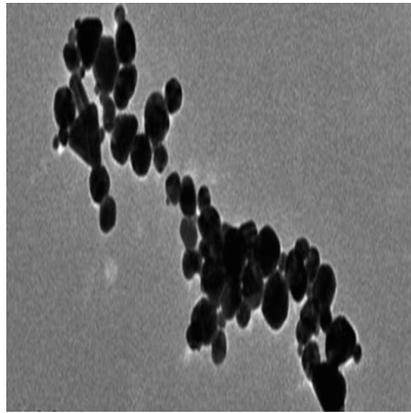
In collaboration with Peking University, NYU Polytechnic School of Engineering professors have been working on a new test strip using gold nanoparticles generated by microplasma that demonstrates immense potential for the early detection of certain heart attacks. The novel method works by sensing a specific marker which is several thousand times higher in patients experiencing myocardial infarction.
