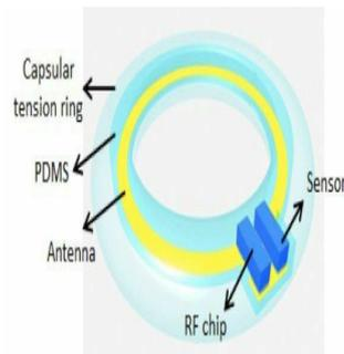
An innovative low-power sensor designed by University of Washington engineers could someday be placed inside a person's eye, tracking otherwise hard-to-measure eye pressure changes and transmitting the data wirelessly via radio frequency waves. Incorporated into an artificial intraocular lens, the sensor would be embedded during cataract surgery, making the replacement lens more functional.
