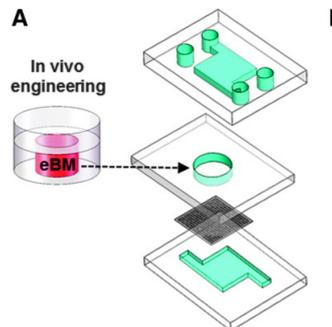
Engineered bone marrow grown in a novel microfluidic chip device responds to damaging radiation exposure followed by treatment with compounds that aid in blood cell recovery in a way that mimics living bone marrow. This new bone marrow-on-a-chip microdevice holds promise for testing and developing improved radiation countermeasures, as described in [Tissue Engineering, Part C, Methods](#), a peer-reviewed journal from Mary Ann Liebert, Inc., publishers.
