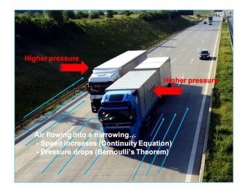
**Figure 1.** The Venturi Effect. According to the continuity equation, when an airflow enters a narrowing, airspeed increases and, according to Bernoulli's theorem, air pressure decreases. As a consequence, air pressure all around is higher compared to the narrowing between the two vehicles, which hence "attract" each other.
