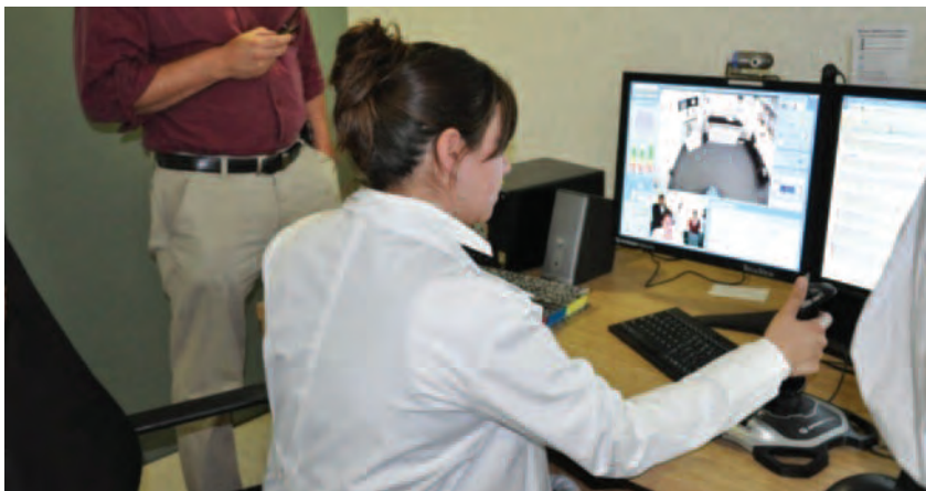
Photo 1. RP-7i® Control Station: Desktop monitor, camera, joystick DT, speakers, keyboard, mouse, microphone and computer. Intensivist at the Maternal and Perinatal University Hospital, Mexico.
