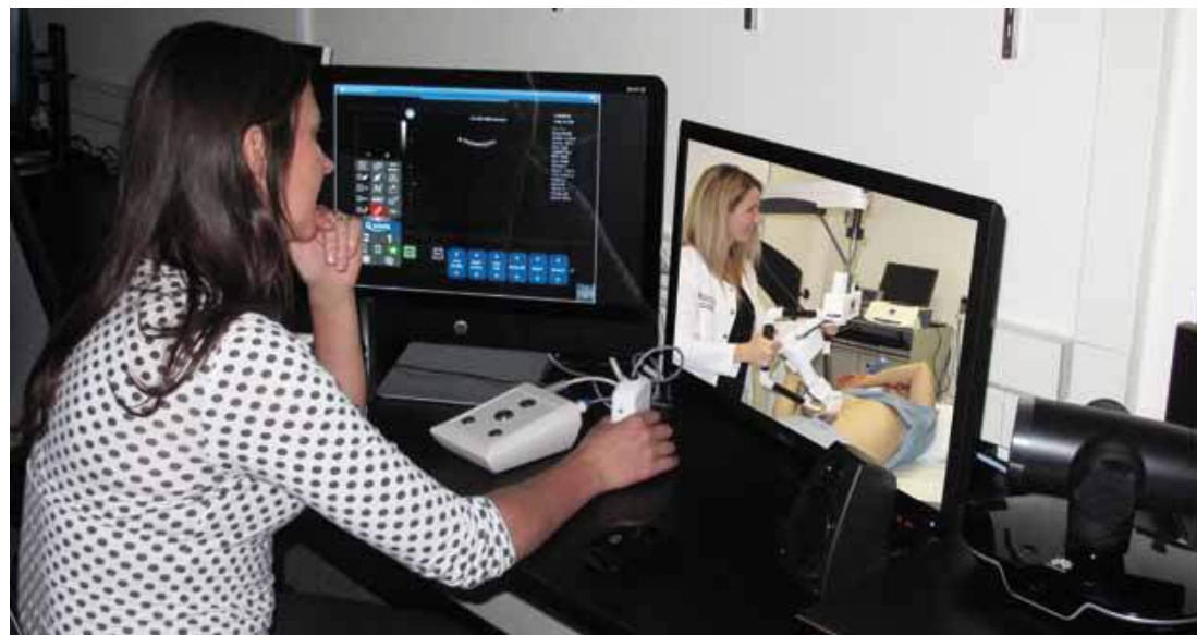
Figure 2. At the central site, a mock transducer enables the sonographer or radiologist to remotely control all settings and fine movements of the transducer, and a touchscreen monitor, which displays the ultrasound system interface, enables the sonographer or radiologist to remotely control all settings. A non-dedicated internet connection connects the two sites, and a videoconferencing system allows for communication between the sonographer, and the patient accompanied by the assistant.
