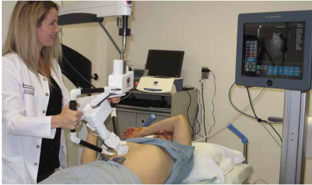
Figure 1. A remote clinic is equipped with an ultrasound unit and robotic arm (MELOD Y Patient System, AdEchoTech, Naveil, France) to which an ultrasound transducer is attached. An assistant with no prior ultrasound experience guides gross placement of the frame for the robotic arm based on instructions from the sonographer or radiologist.
