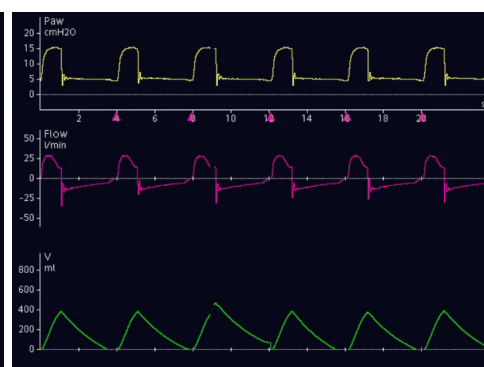
Figure 3b. Improved patient-ventilator interaction with IntelliSync+ activated for cycling-off (simulated patient data)
