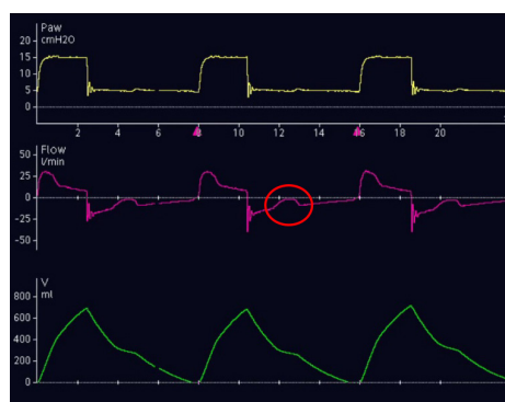
Figure 3a. Late cycling and ineffective efforts with manually set trigger settings (simulated patient data)
